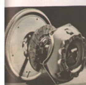
SMOOTH ACTION CLUTCH is easy to operate because clutch pedal spring assists in depressing pedal. Single-plate, dry disc design facilitates gear shifting. The clutch facings are wound in a continuous spiral.
