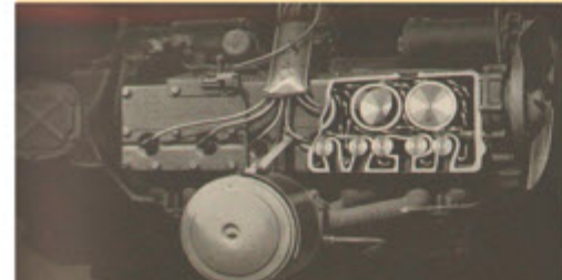
COMPLETELY COOLED CYLINDERS. The cylinder block in Oldsmobile engines is designed so that each cylinder is completely surrounded by cooling water for its entire length. This construction assures positive, uniform cooling and expansion of the cylinders, insuring maximum engine efficiency and performance, and reducing wear to a minimum. Oil temperature is also greatly reduced.
