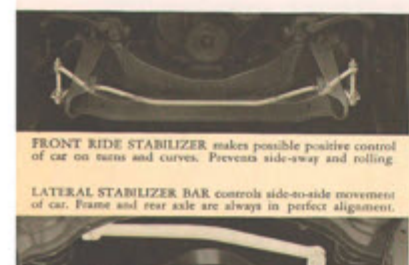
FRONT RIDE STABILIZER makes possible positive control of car on turns and curves. Prevents side-sway and rolling.
