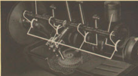
100% FULL-PRESSURE LUBRICATION supplies oil to all vital parts of an Oldsmobile engine. Oil is forced under pressure by a high-capacity, gear-driven pump to crankshaft, camshaft, and connecting rod bearings as well as to the cylinder walls and piston pins. In sub-zero weather, a by-pass permits thick oil to pass directly into the pump without going through the screen.
