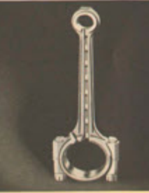
RIFLE-DRILLED CONNECTING RODS. Each Oldsmobile connecting rod is rifle-drilled throughout its entire length to supply oil under pressure to the piston pins and the cylinder walls.
