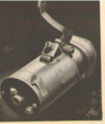
POSITIVE SHIFT STARTER. Flywheel and starter gears engage before motor begins to turn. The plunger-type starter control pedal is isolated from the engine.
