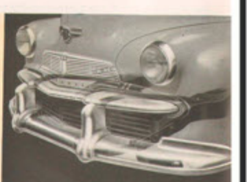
SEALED-BEAM HEADLAMPS insure safe lighting under all driving conditions. Will not deteriorate with use. Lens and reflector are sealed against dirt and water.
