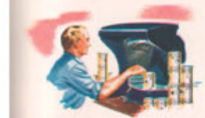
COMPLETELY COOLED CYLINDERS. The cylinder block in Oldsmobile engines is designed so that each cylinder is completely surrounded by cooling water for its entire length. This construction assures positive, uniform cooling and expansion of the cylinders, insuring maximum engine efficiency and performance, and reducing wear to a minimum. Oil temperature is also greatly reduced.
