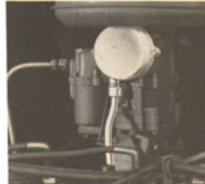
AUTOMATIC CHOKE CONTROL. Quickly adjusts gasoline mixture to any temperature. Prevents gasoline waste caused by over-choking. Makes starting easier under all conditions. Built into carburetor. Has no external linkage.
