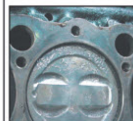
ONLY VISIBLE PISTON DAMAGE
