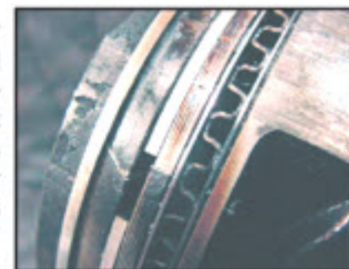
SCOURED & BROKEN PISTON
