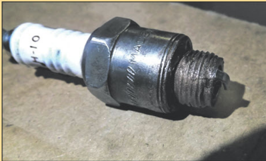
ANTI-SEIZE ON THREADS, NOT ON ELECTRODE
