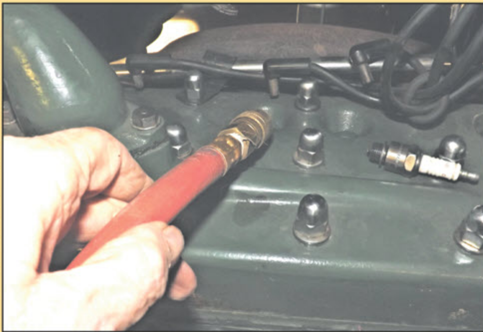
SPARK PLUG HOLES & HEAD BLOWN OFF WITH AIR
