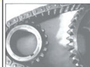
Marks Line Up Straight on a '48 Packard
