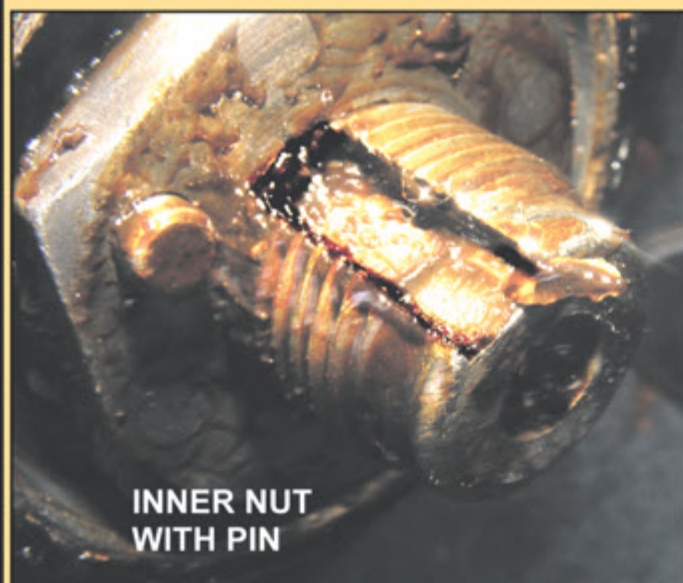
DETAIL OF INNER AXLE NUT WITH LOCK PIN
