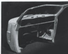
ONE-PIECE COWL ASSEMBLY —An all-steel cowl, welded into one complete unit, gives added strength and rigidity to the entire body structure.
