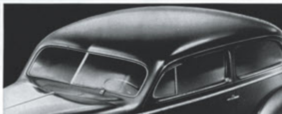
THE FAMOUS FISHER TURRET TOP is made of solid steel and bonded by welding to the big steel body panels to form a continuous, extremely secure steel casing. The roof, itself, is reinforced with rubber-insulated steel cross bows which are welded to the steel inner-body frame.
