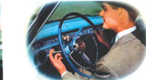
Built-in directional signal equipment is available on all models at extra cost. It operates from a steering post control. Front and rear lamps flash intermittently on either left or right hand turns.
