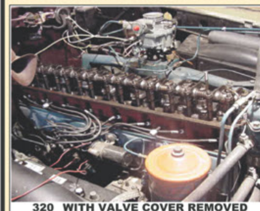
320 WITH VALVE COVER REMOVED
