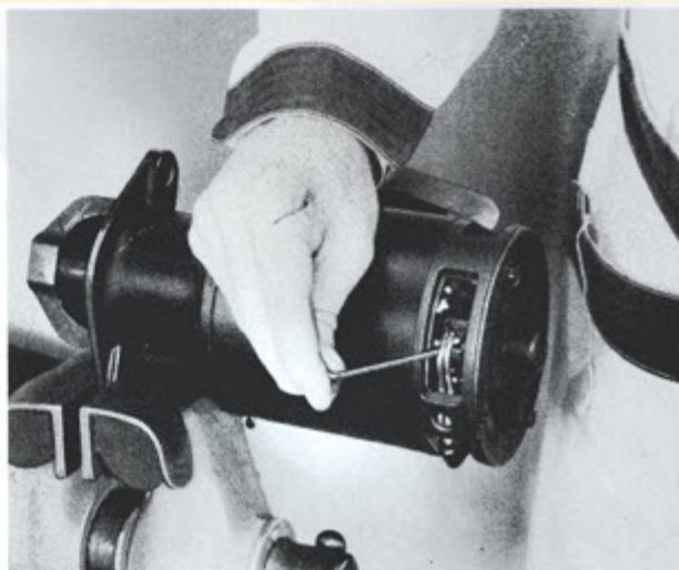
Figure 28—Installing Starter Motor Brushes
