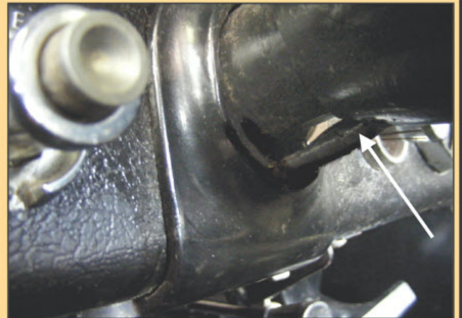
NEW WIRES INSTALLED & WRAPPED WITH ELECTRICAL TAPE GOING UNDER DASH THROUGH STEERING COLUMN COLLAR
