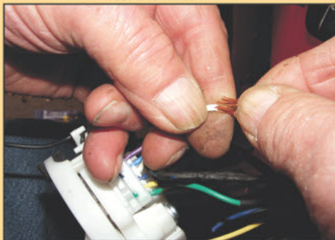
FUSING OLD & NEW WIRES BEFORE SOLDERING
