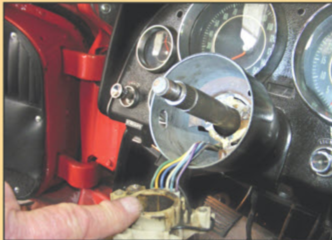
REMOVING TURN SIGNAL/BRAKE LIGHT SWITCH
