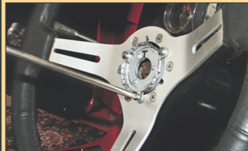
STEERING WHEEL BACK ON WITH 6 PHILLIPS SCREWS (SMALLER WHEEL FOR EASIER EGRESS)
