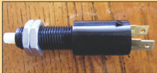
BRAKE LIGHT SWITCH (NUTS ADJUST SWITCH TO TOUCH BRAKE PEDAL)
