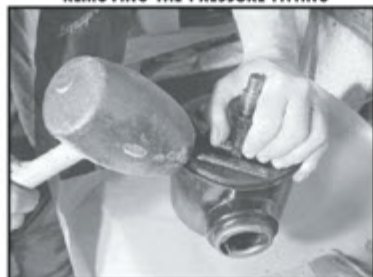
REMOVING THE RESERVOIR
