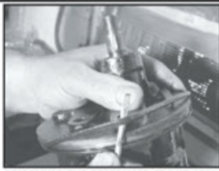
REMOVING THE RESERVOIR FRONT SEAL
