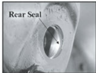
REAR RESERVOIR SEAL CAN BE SEEN
