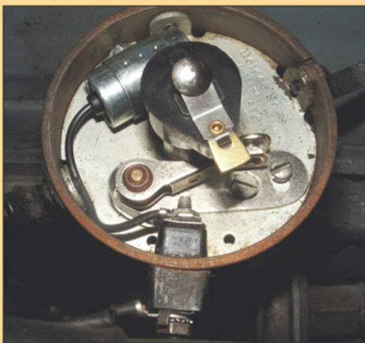
INSIDE OF THE DISTRIBUTOR SHOWING POINTS, ETC.
