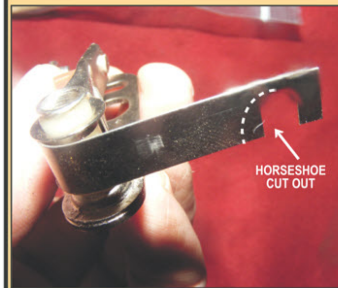
AFTERMARKET POINTS "ARM" THAT GOES TO THE INSULATED TERMINAL WAS TOO LONG!
