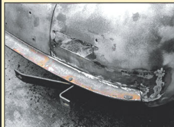
ANY RUST WAS CUT OUT AND NEW PANELS MADE
