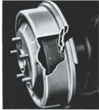
TRIPLE-SEALED BRAKES —Brakes are equipped with three-way seals which prevent dirt, mud and water from reaching the brake mechanism.
