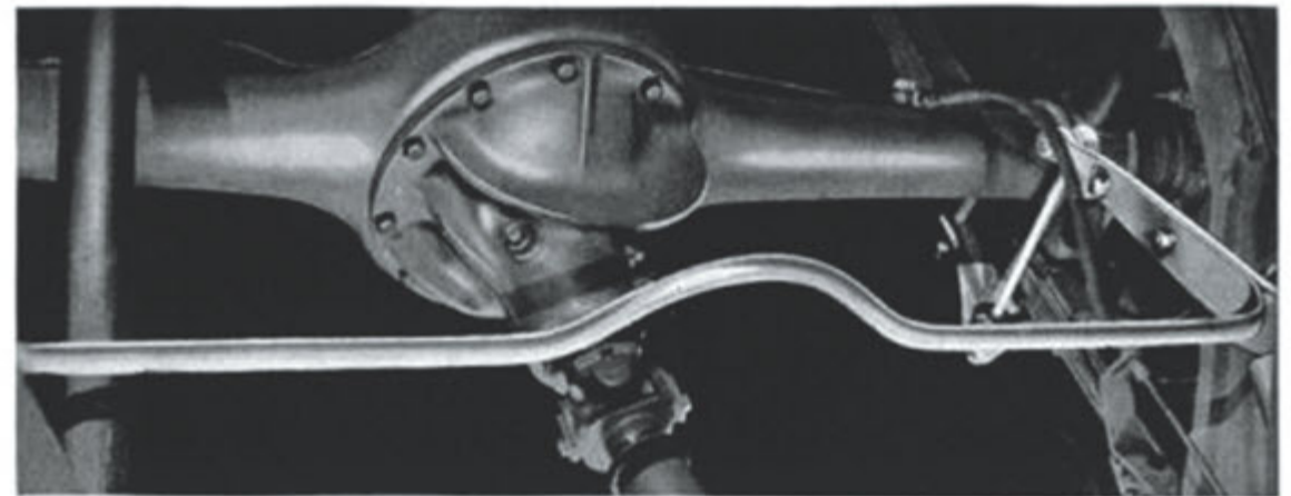
DUAL RIDE STABILIZERS —The Oldsmobile Eight's fine roadability and stability are further improved by two Ride Stabilizers (or sway eliminators), one at the front of the chassis and one at the rear. They eliminate sidesway, lurching, body roll and rear-end wander and result in much better car control at high speeds or when rounding curves. Dual stabilization also gives a steadier ride because its points of application are at both the front and rear ends of the car.
