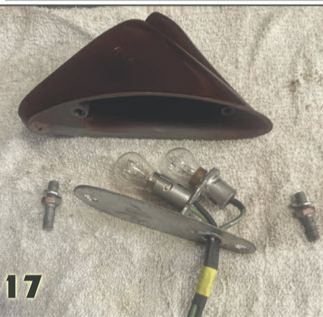
Number 15, 15A This is the light socket that I installed in the tail light bracket.
