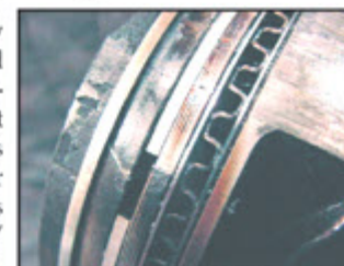
SCOURED & BROKEN PISTON
