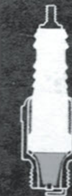
Low insulator seat quickly carries heat from core making a cold plug
