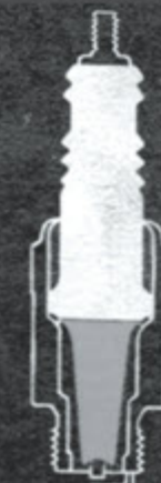
High insulator seat allows core to retain heat making a hot plug.
