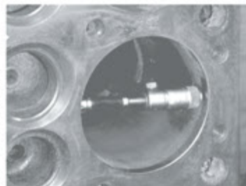
MIKING A CYLINDER BELOW THE RIDGE
