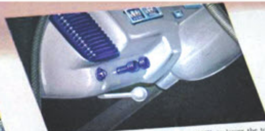
JUST PULL A KNOB ON THE INSTRUMENT PANEL to lower the top—push the knob and it rises instantly when bad weather threatens. Vacuum power is supplied by the engine. Automatic action increases the life of the top, helps to fold neatly when lowered.
