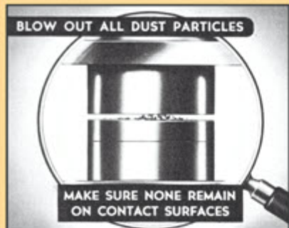
WHEN CONTACTS REQUIRE CLEANING OR REPLACEMENT REMOVE THE DISTRIBUTOR FROM THE ENGINE
