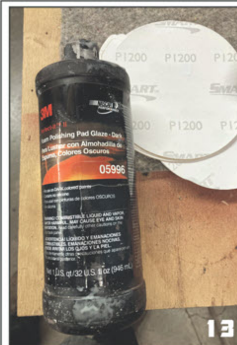
Number 13 Once I have finished COMPOUNDING the car I can finish it off by using my Foam pads. You use the Foam Pads when you put the Glazing compound on. The product is a 3M polish and is Foam Polishing Pad Glaze, 05996. Using a foam pad will take the swirls out of the paint.
