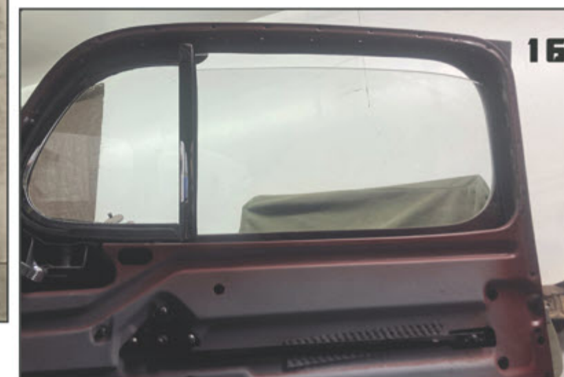
Number 16 In this picture I have the channel in place and rolling the window up and down to check out the fit.
