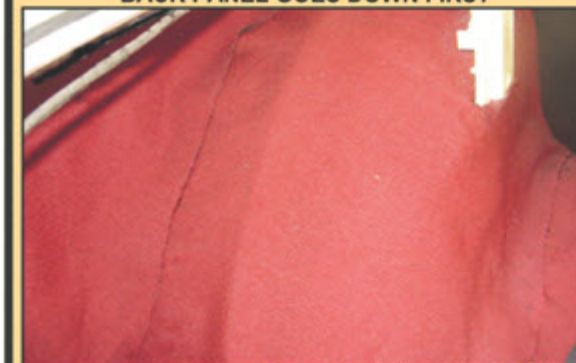
LEFT WHEEL ARCH SHOWING FACTORY CENTER ARCH SEAM
