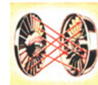
Similarly, liquid is forced against the turbine-like wheel in Fluid Drive. A driving wheel takes the place of gravity.
