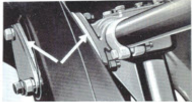
SHOCKLESS STEERING is provided by "cushioning" the steering return mounting in five rubber pads. Road shocks transmitted through the frame are absorbed by the "cushions" . . . "Wheel fight" eliminated.
