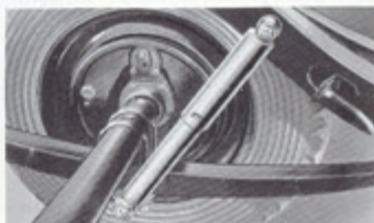
AIRPLANE-TYPE HYDRAULIC SHOCK-ABSORBERS smother the bumps. Double-acting. Low pressure. Automatically adjust themselves to load and road conditions. A cushioned ride!
