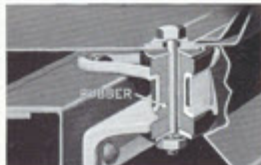
RUBBER FLOAT BODY MOUNTINGS cushion and isolate body from frame. Cut out road rattle and hum. You enjoy a floating ride.
