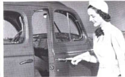
MIN-SLAM DOORS equipped with new Rotary Door Locks may be closed with finger tip pressure. Door slamming is completely eliminated.
