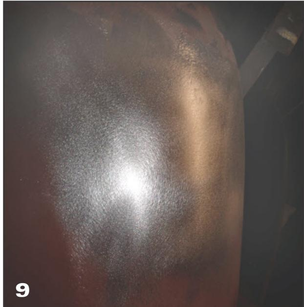
9. The final product as it looks before primer is used. I cleaned up the area and then DA-ed it and it looks like new. It will get a coat of primer when the car is primed and probably in the final analysis needs a little more hand blocking to finish it the way I like it, (but no bondo or lead) and me working about an hour, but like I said before I am rusty, but this is the way they used to do it.
