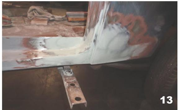
finish off the area. One reason I used the lead was that in this area you could chip the plastic getting in and out of the car. It is ready for the primer and finish blocking of that area.
