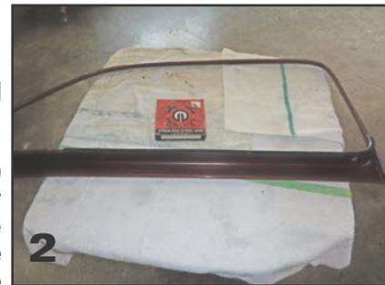
3. This picture shows the new weather strip next to the window frame and the original holes that the factory put in the window frame.
