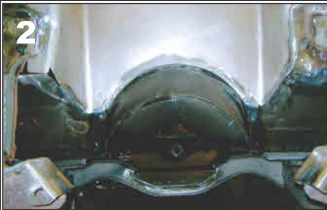
3. This shows the transmission hump from the inside and just how much I had to do in order to install the engine and transmission in the 1951 Ford. This is one of the reasons that I had to make my own firewall panel.
