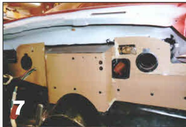
11. This is the completed panel ready to install on the firewall. When I installed the panel on the firewall I used a 3/8 hole saw to add a hole where I needed to run a wire thru the panel and it worked very nicely.
