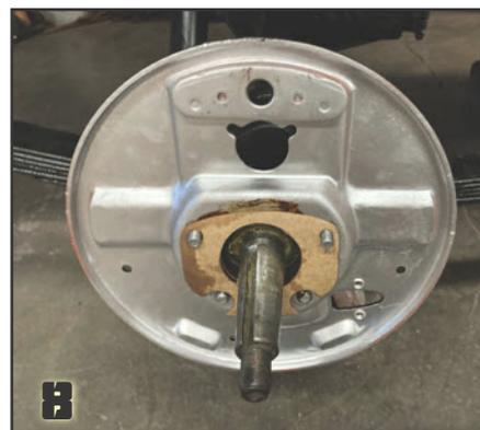
on the backing plate before I put the gasket on. One note on using original gaskets, if it is old and dry I will soak it in water before I put it on the car.
