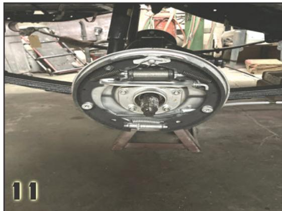
thing, when you remove the return springs the ends get bent out so squeeze the ends back where they belong when you finish installing the springs.
