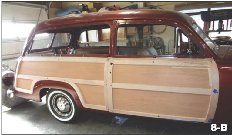
8-B. •This is another picture of the two panels on the car and showing how I pulled the rear in to fit everything.
