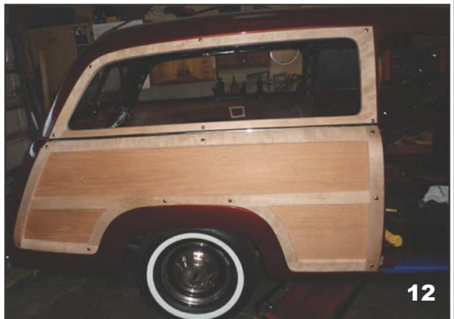
Now that I have all the wood and the panels installed, I can take it all apart again and remove all the screws. • I get the job of sanding all my fingerprints and pencil marks off and making it ready for the varnish. • I have more respect for the work my body builder did when he built our 1941 120 Packard station wagon. • It is a lot of work but the end product is BEAUTIFUL.
