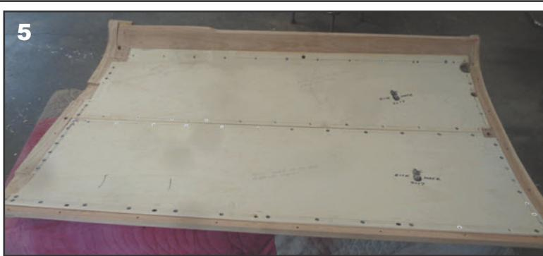
5. The whole door has had the wood inserts installed and ready to put on the car to check for clearance problems. I chose to put the screws every 4 inches for the center, as that was Rick's suggestion, and I used 2 inches on the side as that was what I thought I liked best.
