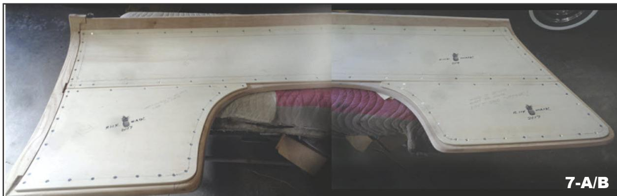
7. A/ B These are the rear inserts, which have all been drilled and screwed into the rear section (the lower quarter section of the quarter panel).
