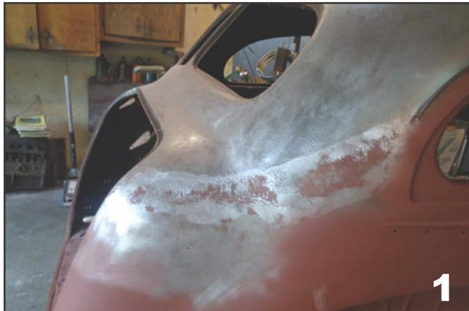
Bondo, which is still around. Today's plastic fillers are great, but quite frankly there are places to use lead and the body seams are a good example. The seam will probably have up to a  $\frac{1}{4}$  inch of lead in the repair. The lead lasted 70 years, but it had cracks and the crack went all the way to the body.
