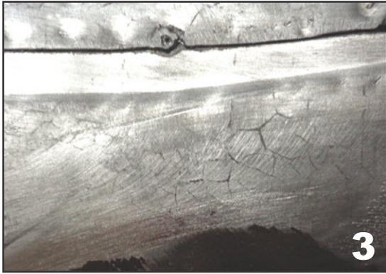
3. This is a picture that shows where I have melted all the lead off the seam area and completely wiped the area with a piece of steel wool. Where there are cracks in the lead, the cracks went all the way to the body and left rust spots in the metal. These areas are now clearly visible.
