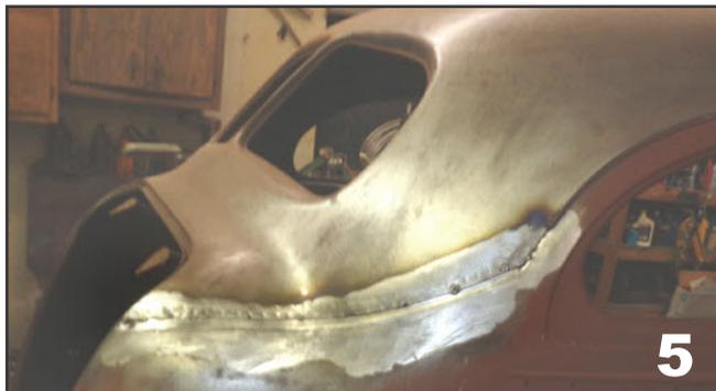
grind or sand to get good clean metal to prep. 5A & 5B. These two pictures show a close-up of where I am cleaning and prepping the area. You can see the corrosion around the factory welds that I have to further clean up by grinding..
