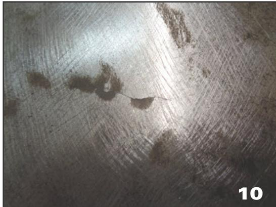
10. I discovered this crack in the roof top in an area that I had just begun to work. I use a flat file to start with when I start a new section to see what is high and low and in doing so I found this crack. I have used the flat file and you can see my file marks and can see the high and lows in the crack area and at the top of the crack
