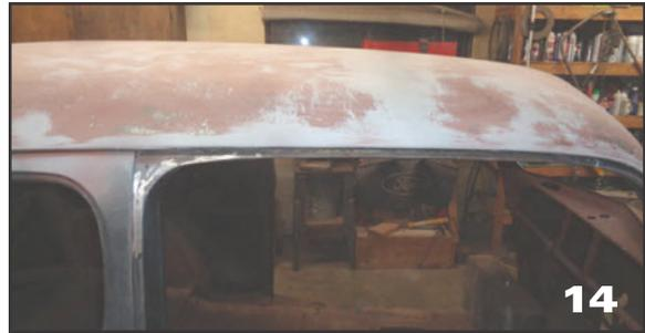
15. This picture is one that shows how I have sanded lightly to find high and lows. This is after I have been picking and filing the top and now put paint on it to find the problems. I have several different lengths of DURA BLOCK brand blocks that are flexible and contour nicely to the top of the car. I used the 20 inch block on this area. The difference in color of the gray primer shows the lows and high spots.
