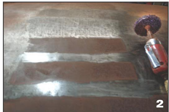
the top a section at a time. VERY tedious using the stripping wheel and you get very dirty doing this. But I am getting it down to bare metal.
