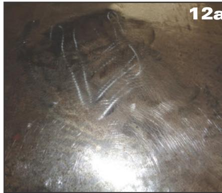
I have only showed a couple examples of using the flat file and working the roof to get it fixed. Each section that I worked on required a lot of work and then once I got the roof reasonably done then I used my two color primer to then block sand the
