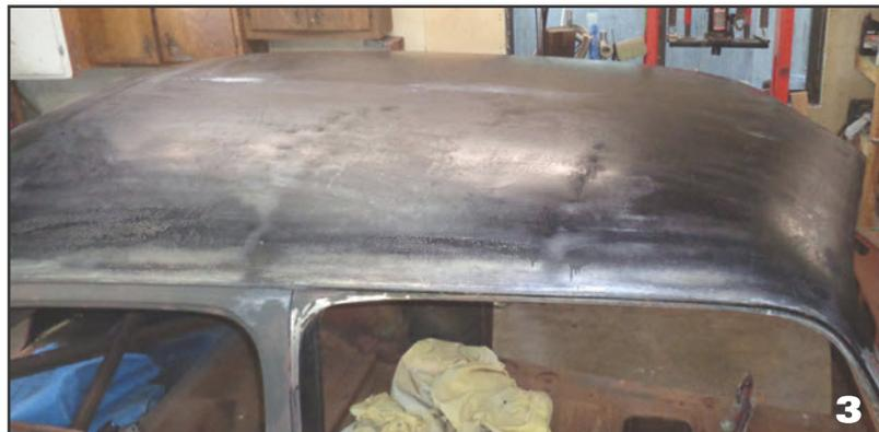
3. The top after I have finished stripping the rust off it and I have DA'ed the whole top.
