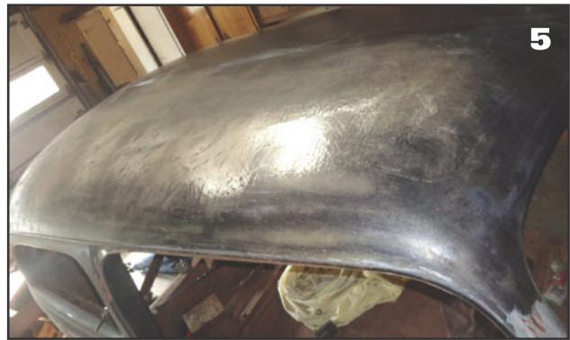
6. I have sprayed the whole roof with Red primer so that I can start figuring out how bad the dents in the top are.
