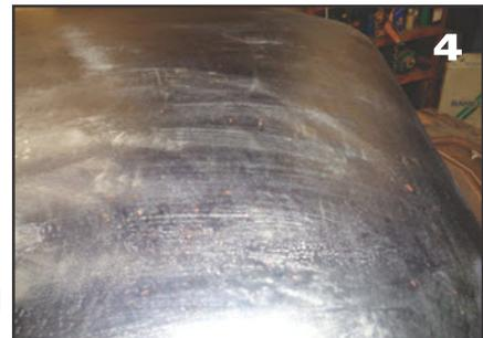
4. close up of the top showing how it cleaned up and I have sprayed the chemical Permatex Rust treatment on it.
