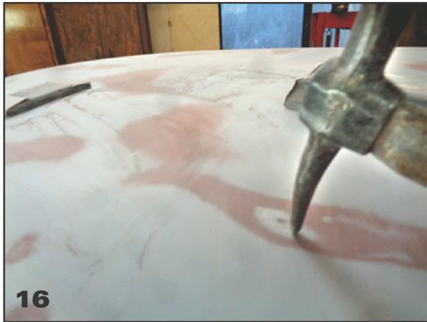
down and I will also be lightly hitting the area up that is low from underneath. ALWAYS use a gentle taps with the hammer.
